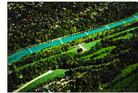
The series of cross-river sills built into the river every 200 metres prevented the straightened river from eroding away at its bed and made it impossible for the fish to embark on spawning migrations. In periods of low or medium water flow, they turned the Isar into a chain of dammed ponds.
